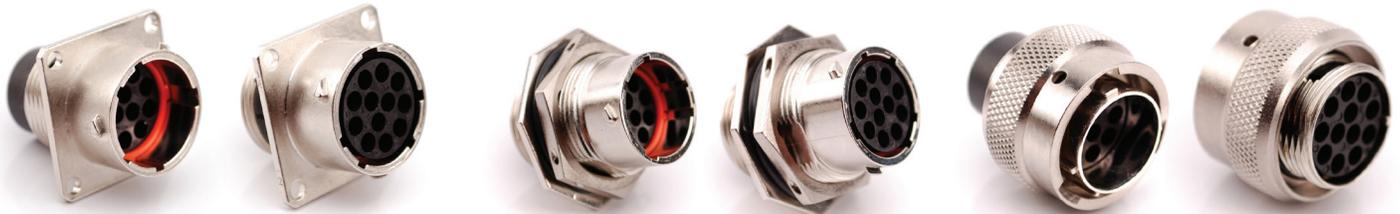
RT360™ industrial circular connectors are multiway connector available in 6 shell sizes and 22 insert arrangements with a variety of wire gauge options. RT360 industrial circular connectors were designed to be intermateable with other industry standard connectors, such as the Souriau TRIM TRIO UTG and UTP industrial connector families and Cannon Trident series.
