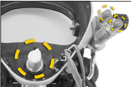
3) Cap or plug the Regulator Mount Tube, One Way Valve Adapter and Emergency Valve Inlet to prevent debris from entering during drilling
