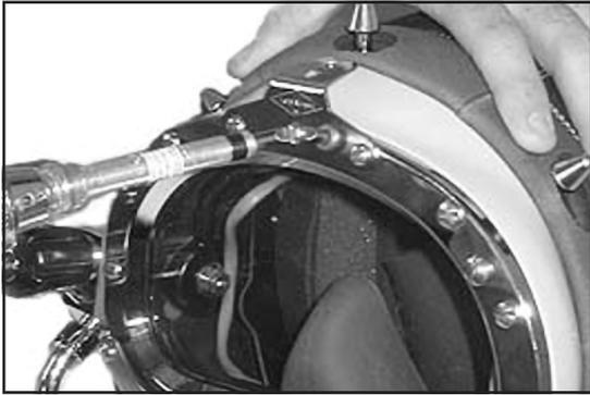
13) Install the Top Band Keeper Mount onto the front of the Port Retainer using three Screws (P/N 530-040) and tighten them with a Torque Screwdriver to 12 inch pounds.
