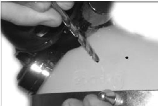
4) To Drill the holes accurately use a Drill Start or twist the Drill Bit by hand to start the holes first to prevent the drill from wandering. Use a #10 (0.1935") Drill and carefully drill the two holes.
