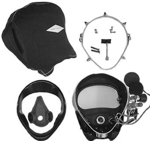
The following parts must be removed from your KMB 18/28. Refer to the KMB 18/28 Manual which can also be found online at [www.kirbymorgan.com](#) for removal procedures. Remove the Head Harness (Spider), Hood, Top & Bottom Bands, Comfort Insert (KMB 18's Only) Nose Block Device, Oral Nasal and the Three Top Port Retainer Screws. Inspect and replace if necessary parts that will be reused for the installation of the new Hood & Band Keepers.
