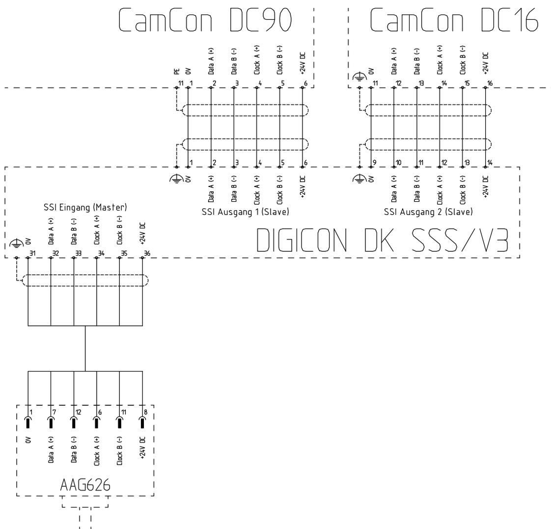
7.2. Connection example for Listen - mode of a Multiturn – Encoder with 4096\*4096 (24 Bit)
