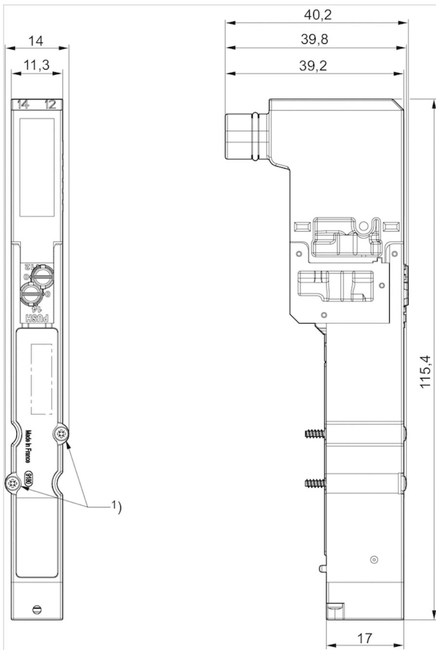
1) Mounting screw: X-slot DIN EN ISO 4757-Z0
