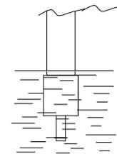
The contact is OPEN when the float is in the liquid
