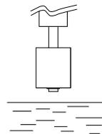
The contact is CLOSED when float is above the liquid level.
