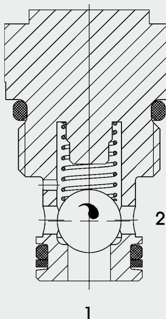
The check valve RVM06020 is a direct-acting, spring-loaded ball poppet valve. When there is no flow through the valve, the spring holds the ball in the closed position and therefore shuts off port 2 from port 1. The valve opens when the pressure at port 1 is higher than the pressure at port 2, including the pressure created by the spring force.
