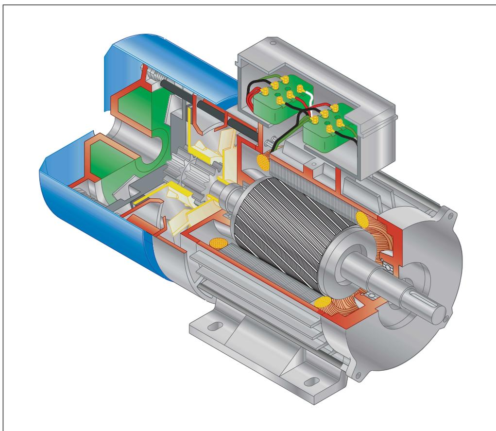
Coel motors are closed and externally ventilated. The brake groups and all the motor parts are made by Coel. The brake group is supplied on series with "3ph. AC" electromagnet but DC version is also available on request. The F series motors can be driven by inverter but in this case the brake supply must be separated from the one of the motor.
