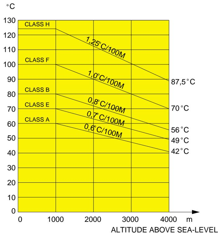
Limits in excess temperatures depending on the altitude at installation for trials carried out at altitudes less than 1000m, for machinery meant for installation at up to 4000m (coolant temperature 40°C).
