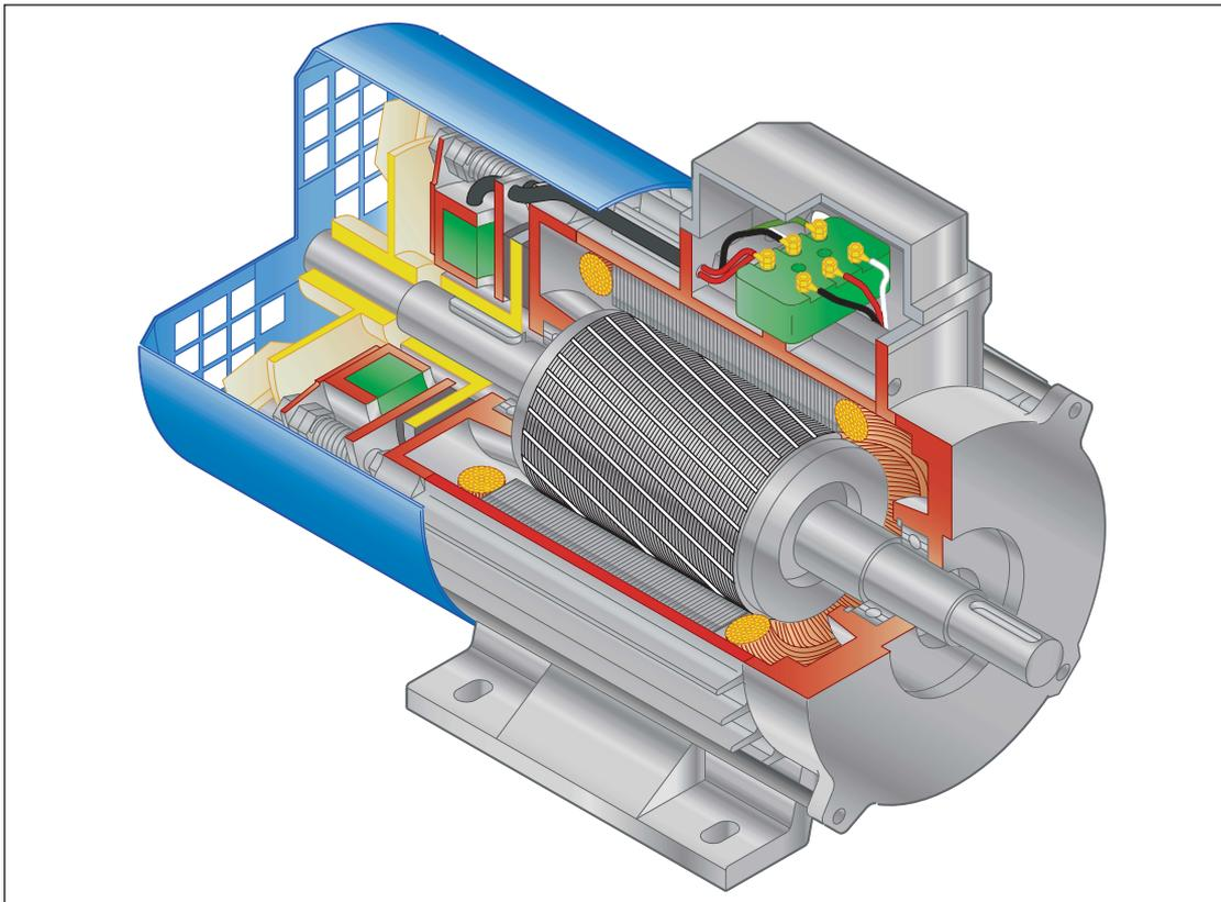
FK motors are fitted with DC brake as standard. The motor operates with very low noise and it's suitable also for inverter duty.
