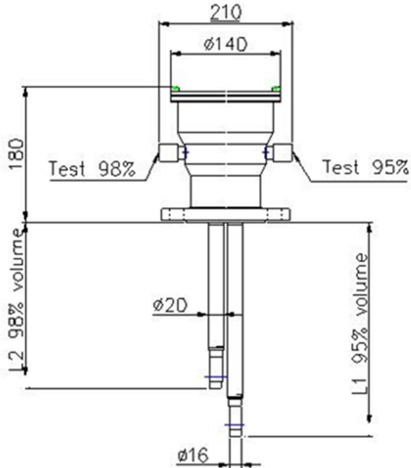
TLA level switch with DN50 flange.
