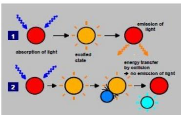
Principle of dynamic quenching of luminescence by molecular oxygen
