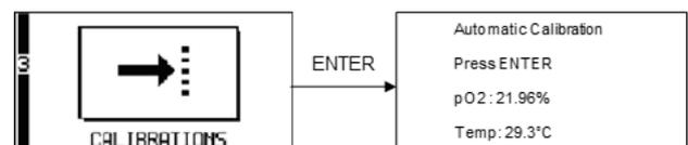
Wait for the values ( $O_2$  and  $^{\circ}C$ ) to stabilize, then press ENTER; if the procedure is successful the display will show "Calibration OK"
