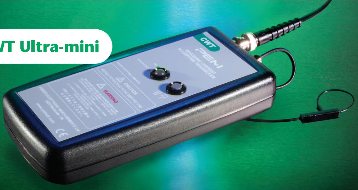
The CWT Ultra-mini has an extremely thin, clip-around Rogowski coil of typically 1.6mm cross-section. Such a thin coil enables currents to be measured in the most difficult to reach parts of a power electronic converter with negligible disruption to the circuit under test.
