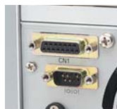
Upper: D-SUB connector Under: RS-232C
