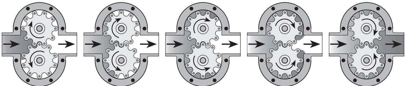
Flow Technology positive displacement flowmeters use two rotating impellers driven by the flowing liquid. Magnets imbedded in the impellers activate a non-intrusive sensor which generates a pulsed output signal. Each pulse represents a known volume of liquid that is captured in between the lobes of the impellers. A K-factor converts the pulses into engineering units for remote data collection and digital display.
