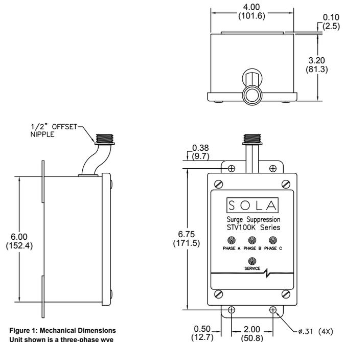
Figure 1: Mechanical Dimensions
