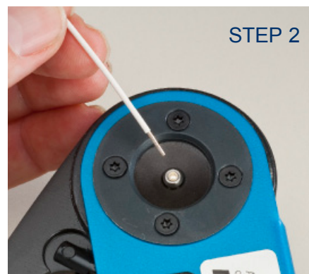
INSERT PRE-STRIPPED WIRE
