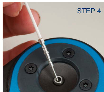
REMOVE TERMINATED WIRE ASSEMBLY
