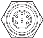
6-pin RSFLV-66 Turck Banner connector pin 2 +ve pin 3 -ve
