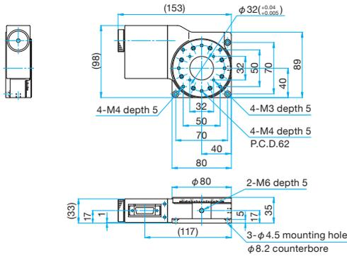
**OSMS-120YAW** Hexagon socket head cap screw M6×10...3 screws
