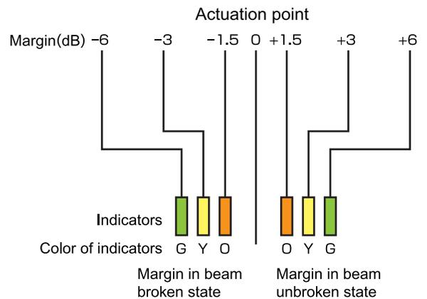
For example, when green indicators for both beam unbroken and beam broken states illuminate, the sensitivity-set-points in both beam unbroken and beam broken states are set with  $\pm 6$  dB or more margins to the actuation point.
