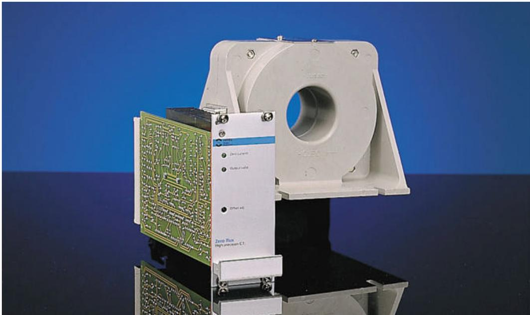
The STACC is a high precision DC current measuring system based on the zero-flux principle for currents up to 6000 A.
